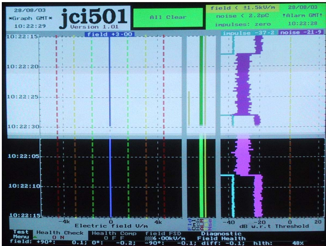
Operation in 'test mode' showing operational health modulation signals on noise and impulse channels and start of unsatisfactory indicator of fieldmeter health while its sensing aperture was shielded.
