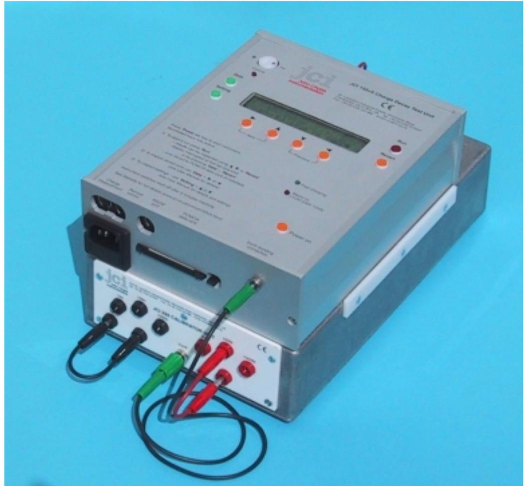
JCI 155v5 Charge Decay Test Unit on JCI 255 Calibrator Unit
