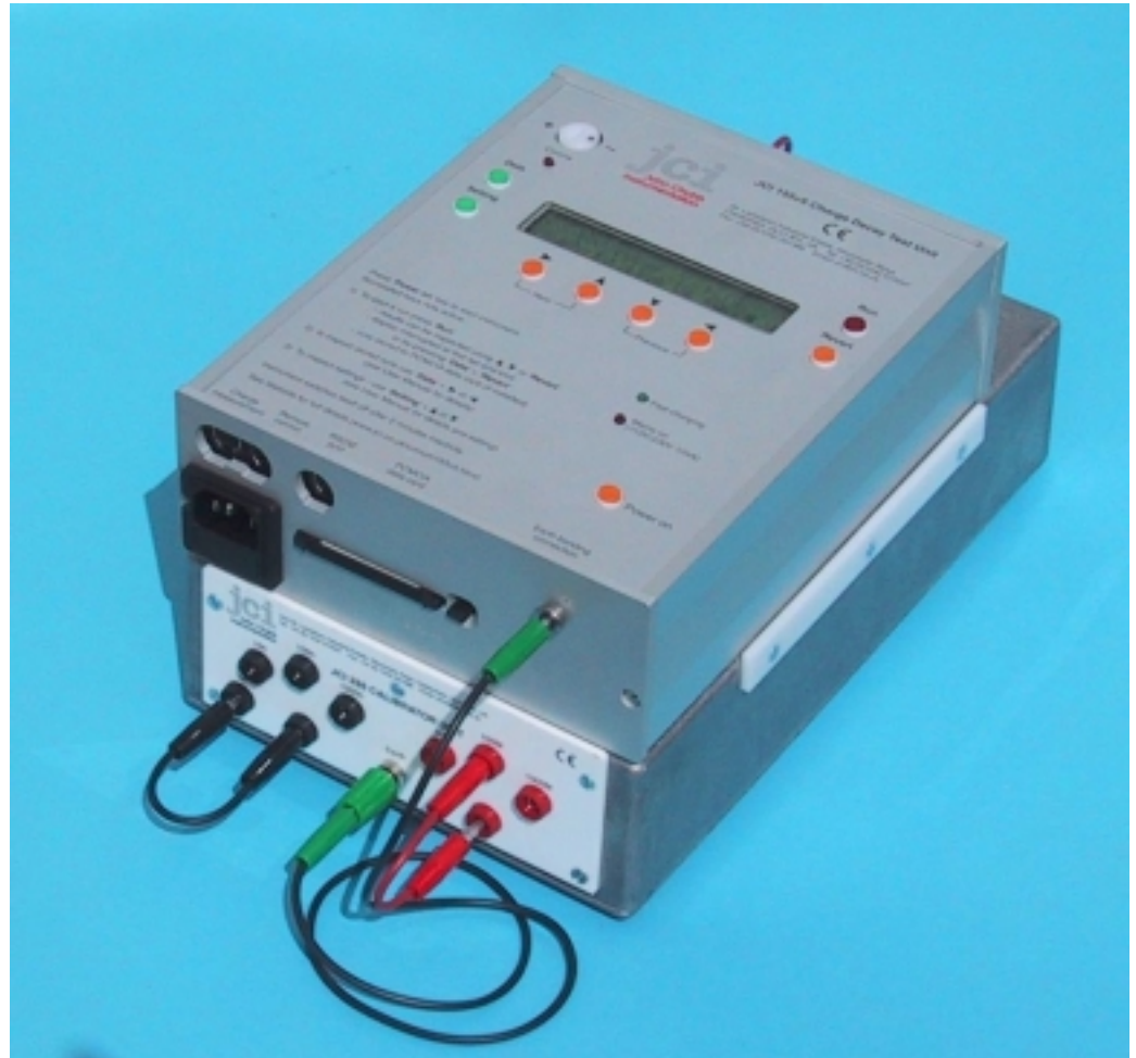
JCI 155v5 Charge Decay Test Unit on JCI 255 Calibrator Unit
