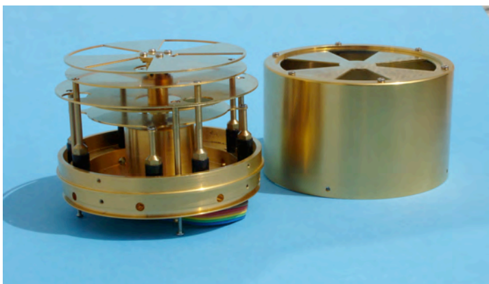
Internal structure of JCI 131 electrostatic fieldmeter
