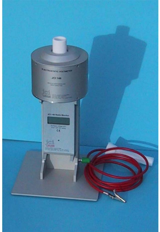
The JCI 140 Static Monitor is easily removable from the mechanical arrangement and can be used in its own right for other measurement purposes.
