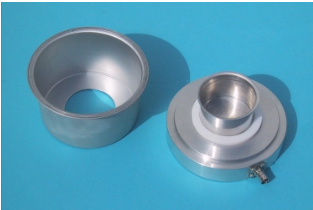
JCI 150 Faraday Pail: baseplate, BNC connector, insulation, pail and shield
