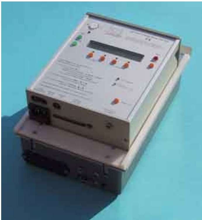
JCI 155v5 Charge Decay Test Unit on JCI 176 Charge Measuring Sample Support
