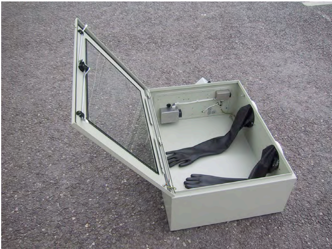
Inside of JCI 191 Controlled Humidity Test Chamber
