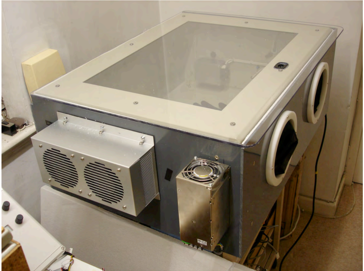
JCI 191C showing power supply and thermoelectric cooler units and overall thermal insulation
