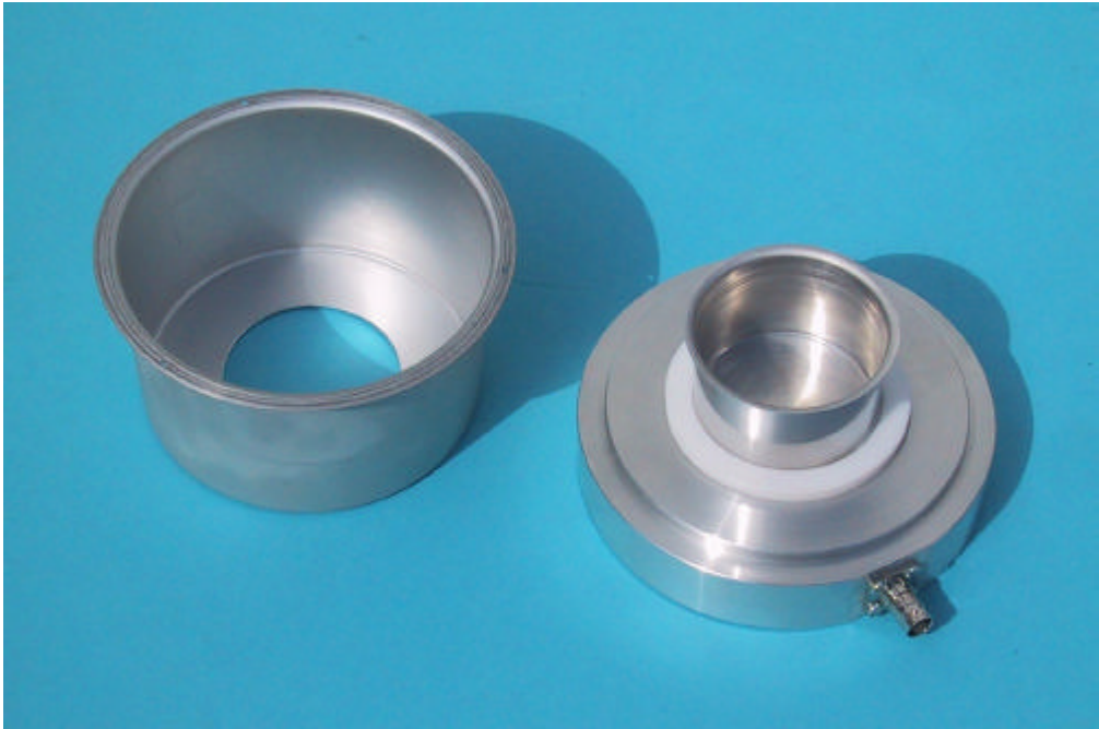
Figure 2: JCI 150 Faraday Pail: baseplate, BNC connector, insulation, pail and shield
