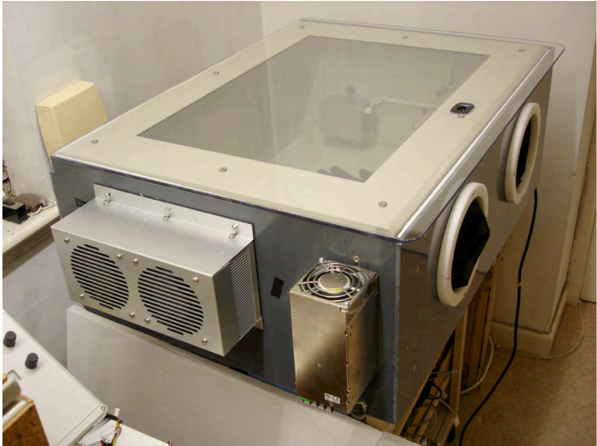
Figure 3: JCI 191C showing power supply and thermoelectric cooler units and overall thermal insulation
