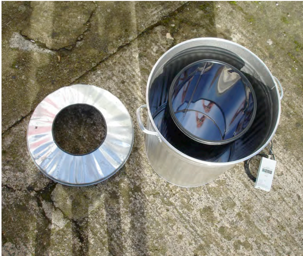
Figure 2: JCI 247 with shield off to show removable pail
