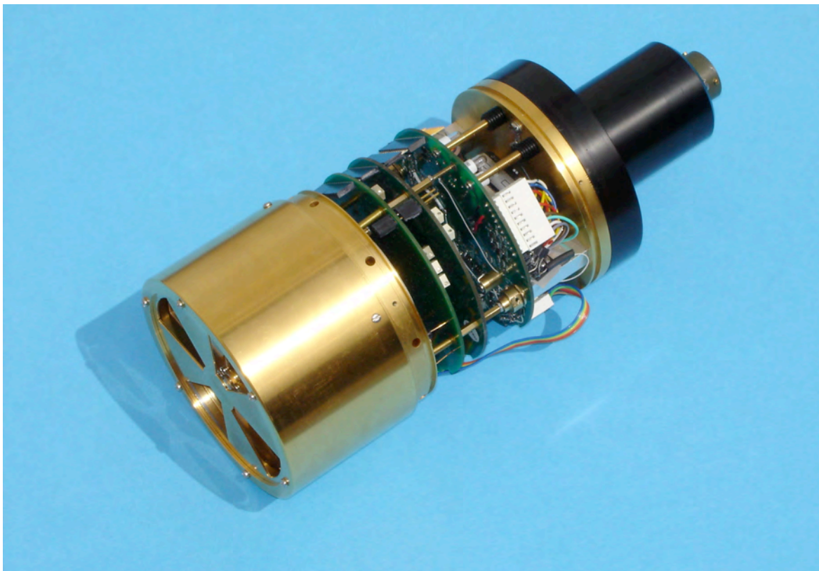
Figure 2: Assembly of JCI 131 fieldmeter - with rear casing removed to show mounting of fieldmeter, operational health and power supply circuit boards
