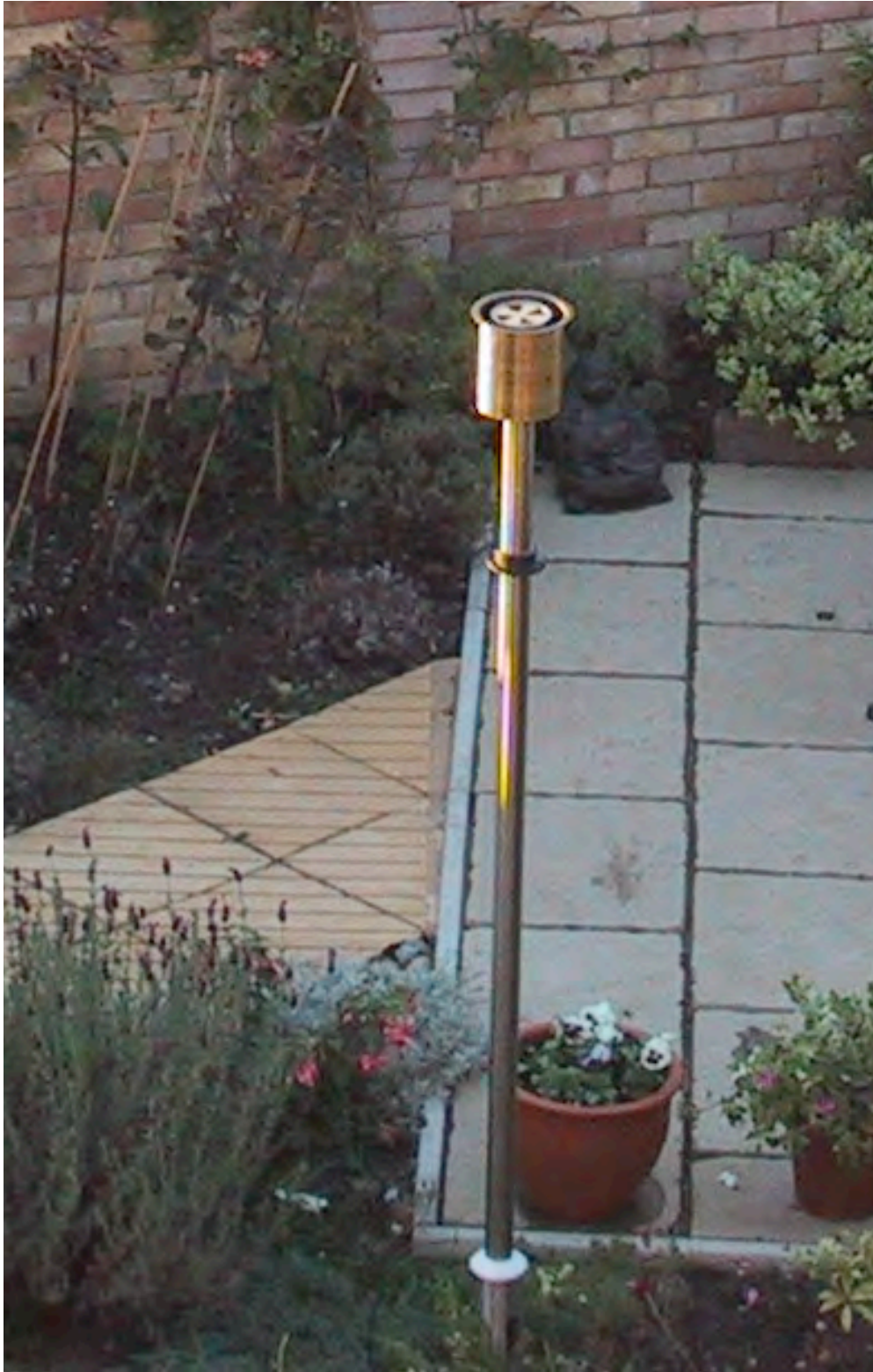
Figure 3: JCI 131 fieldmeter on mounting pole with operational health shield fitted
